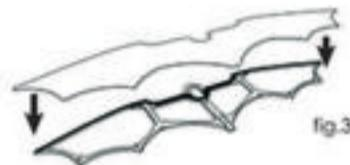
**Attach the fabric to the surface of the glider (Figure 3 and Figure 4)**
